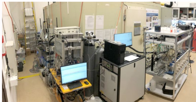
Experimental set-up of PAM OFR-Chamber system to study volatile organic compound oxidation and secondary organic aerosol formation 實驗裝置，用於研究揮發性有機物的氧化和二次有機氣溶膠的形成
